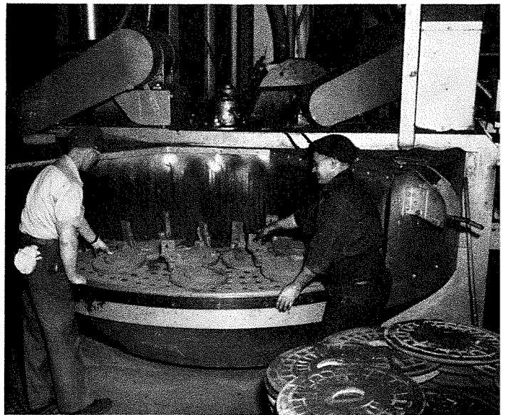
10' Wheelabrator Plain Table installed in their foundry. This old textile machine manufacturer operates the largest foundry in New England.
